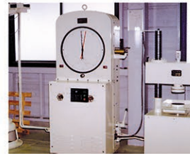
Hydraulic compression testing machine
